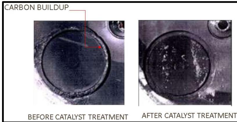
In the photograph above you can see the result of using one of our programs. This is the cylinder head of a truck, in it you can see the carbon build up and then the result of using the catalyst. The carbon deposits are removed because the catalyst has involved them in a chemical reaction during combustion thus removing them from the valve. It is important to point out that this is not a detergent action but the normal action of the catalyst behaving normally.
